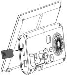
To insert a memory card, push the card firmly into the memory card slot in the direction as indicated above, with the metal contacts of the card facing towards the picture frame
